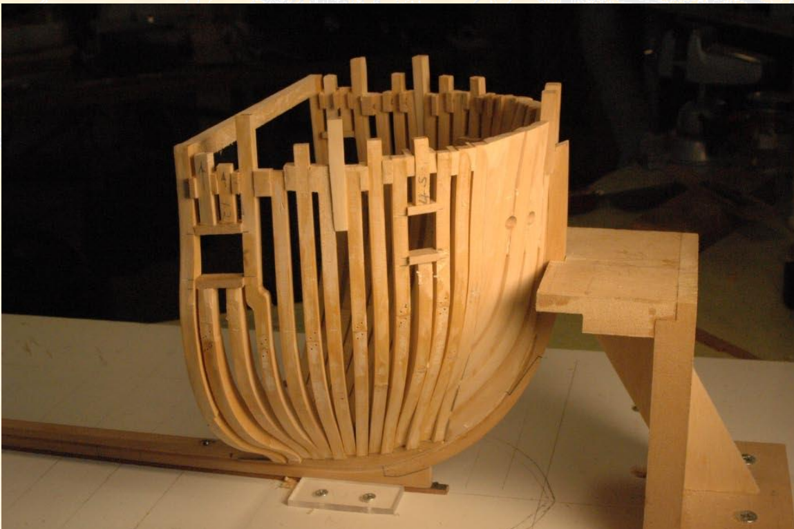
Figure 20 — all forward cant frames installed
