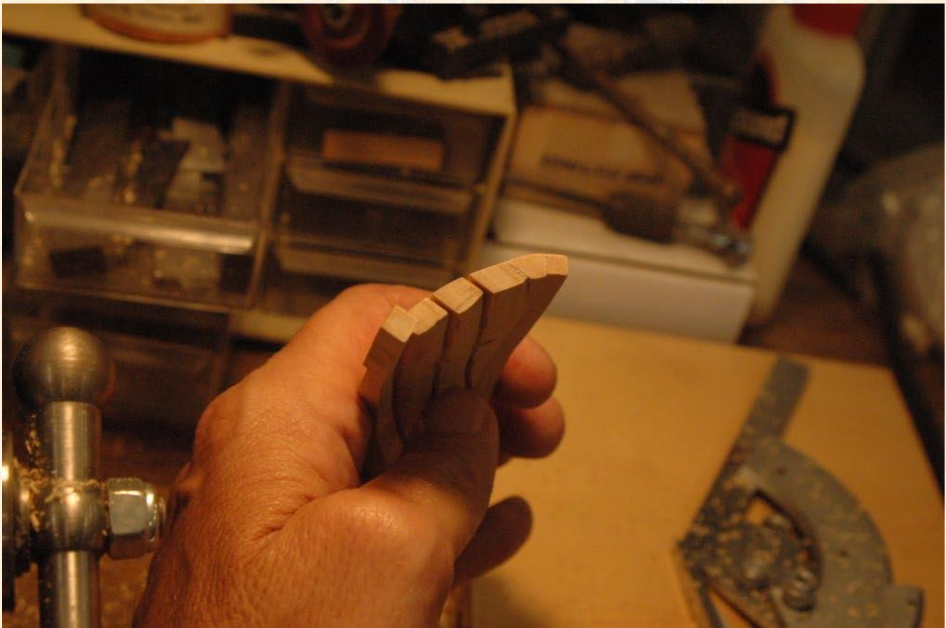
Figure 13 — starboard hawse timbers
