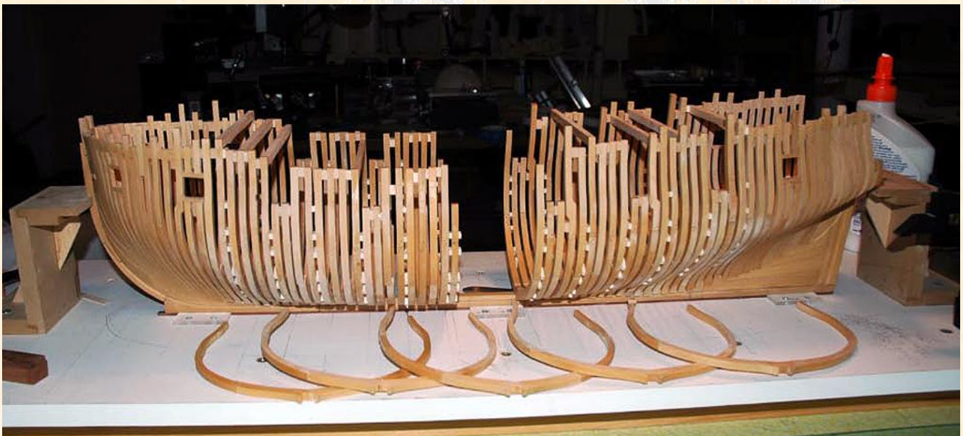
Figure 3 — framing advancing towards center
