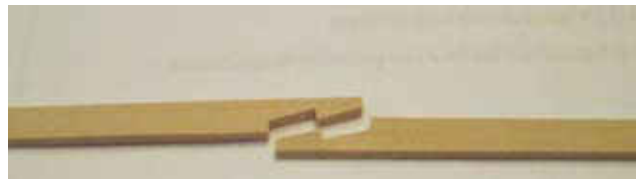
Mike showed his model of HMS Fly and demonstrated how he made the hook/scarph joint for the wales.
