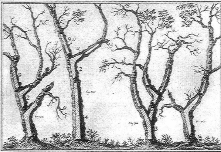
Illustration from a book for naval architects, published in 1789. It served as a guide to shipbuilders, who chose trees that would yield pieces of the desired shape. In the 18th cent. so much wood was used in building English ships that the British Isles were virtually deforested and timbers were imported from America. The cross sections at the right show how the pieces were fitted together in constructing a hull.
