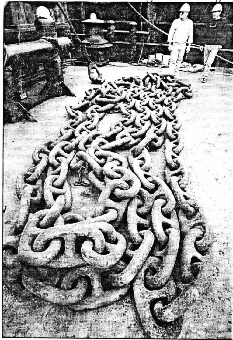
Catenary chain on after deck of Sea Victory.
