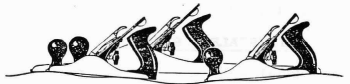
A short plane follows the shape of the wood as a small boat rides over the waves and into the hollows between. A longer plane does not follow the hollows.
