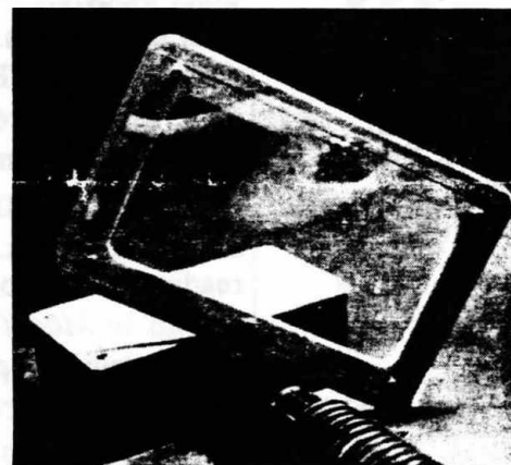
4 Screw a sheet of 20- or 30-gauge plastic to the plywood frame, and you're ready to vacuum-form a part.
