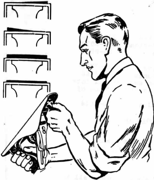
Sight along the bottom of the plane. Let the blade project a hair's breadth and set the corners evenly.
