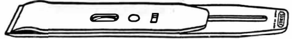
Set the cap iron of the double blade near the cutting edge for hard wood—farther back for soft wood—or about \frac{1}{8} " or the thickness of a dime.
