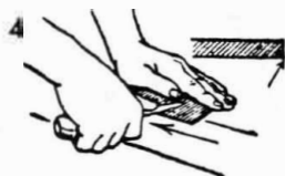
4. Draw the edge with three or four firm strokes of the burnisher held flat on the scraper.
