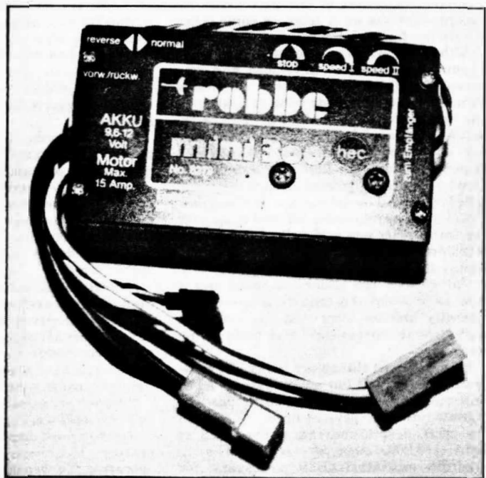
Above: another two function outfit from a different distributor, the Sanwa FM system, distributed by Irvine. All of today's sets are extremely reliable and styling and feel of the transmitter plays a large part in deciding on any particular make. Right: an electronic speed controller for scale and fast electric models. This one is distributed by Cougar Craft and will operate on most modern systems.
