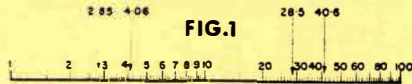
THIS IS A TYPICAL SCALE DRAWN ABOUT ONE THIRD FULL SIZE A 12 INCH SLIDE RULE IS MORE FINELY DIVIDED EG THERE ARE FIFTY DIVISIONS BETWEEN '1' AND '2'
