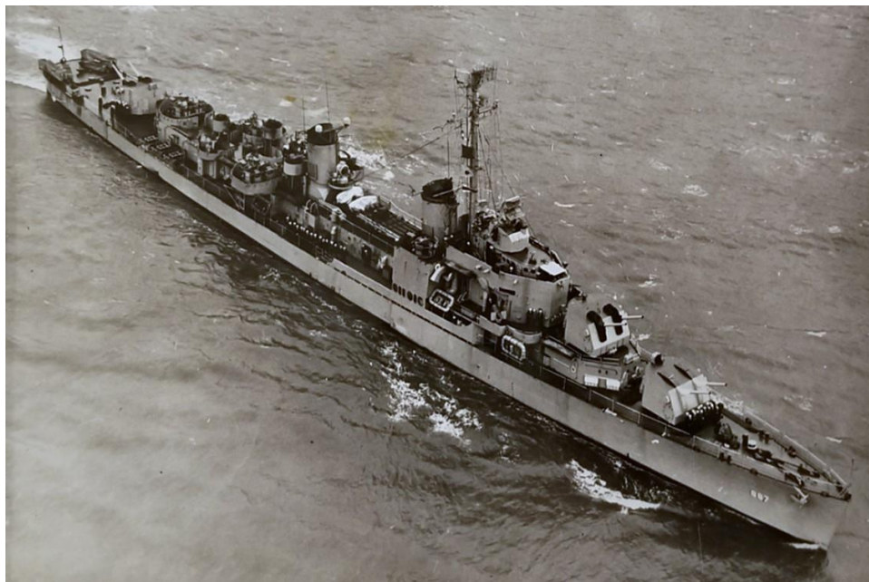
BRINKLEY BASS "as built" with a quad 40mm gun mount replacing aft torpedo tubes of the original design to combat Kamikaze aircraft threats late in World War II. Oct 1945 photo from 1st Commanding Officer CDR Philip Wallace Winston, USN
