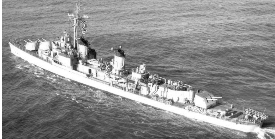
BRINKLEY BASS in the mid-1950s with tripod mast for heavier radars and 3"/50 gun mounts replacing 40mm and 20mm AAW batteries from http://www.navsource.org/archives/05/pix1/0588712.jpg
